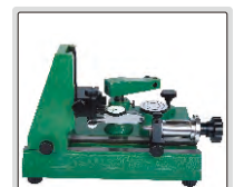
inspect accuracy of test indicators
