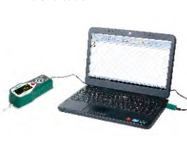
via SPC cable
